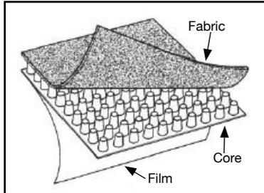
The Drain Max 220 Series is designed for use with the Drain Max waterproofing systems in vertical installations.
